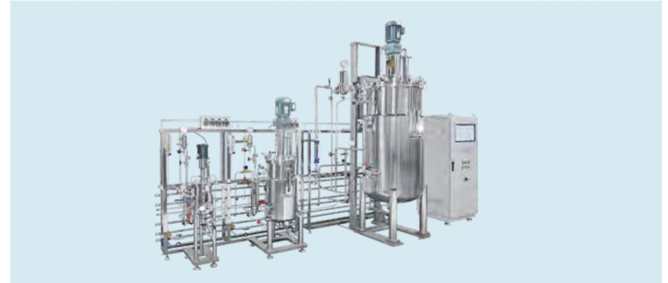
YC-JSMS-X can be equipped with multi-step seed vessels, which is a powerful assistant for process research, development and optimization. Saving labor and time for rapid process validation.
