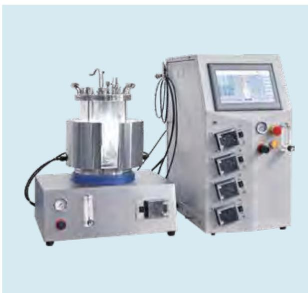
YC-JGG is laboratory benchtop illumination bioreactor. The lampshade surrounds the glass vessel without taking up extra space, and is more suitable for plant cell growth.
