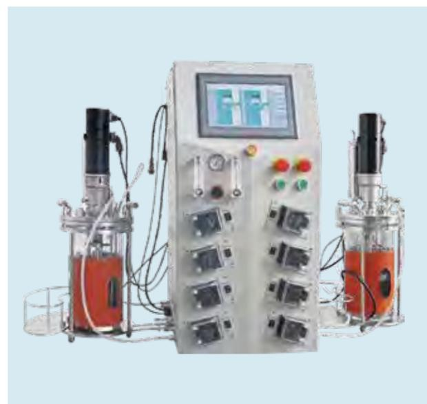
YC-JGD controls two vessels by one controller, which is universal with YC-JG/CG series glass vessels, so replacement is not limited, and save more time and space.
