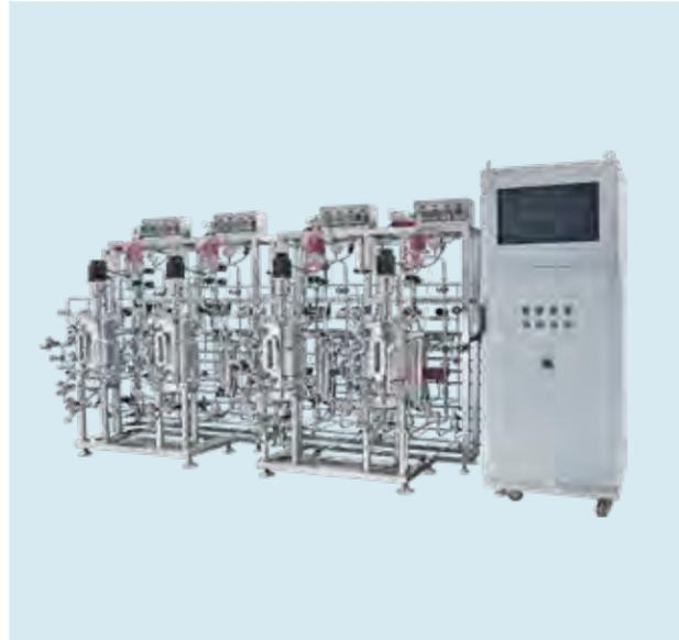
YC-JSM-X controls multiple vessels of the same size by one controller, which can achieve rapid process verification. It is suitable for contrast experiments.
