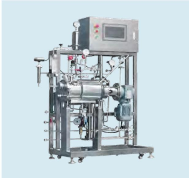
YC-SS is equipped with a rolling axis vessel, and suitable for the transition experiment of solid fermentation from laboratory scale to production.
