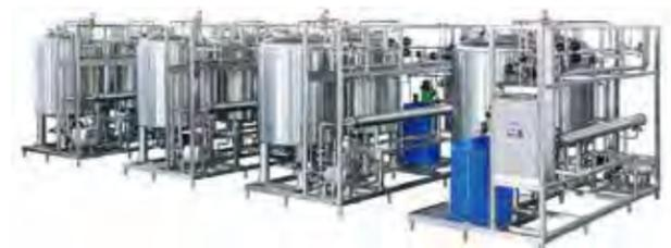
For automated cleaning procedures, a CIP system may be used with SIP fermentation system. Additional valves, connections, and spray-balls will be installed to allow connection of your own CIP system.
