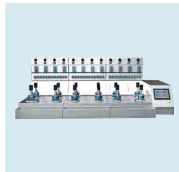
YC-MJG-X is a miniature parallel bioreactor with integrated design and more precise configuration, which helps scientists to manage more experiments at the same time.
