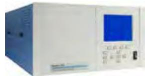
The CO<sub>2</sub> / O<sub>2</sub> off-gas analyzer provides real-time measurement of carbon dioxide and oxygen concentration of the bioreactor exhaust gas. The CO<sub>2</sub> concentration is determined by a self-calibrating non-dispersion infrared sensor, while an electrochemical sensor monitors the oxygen concentration. Users can monitor metabolism and analyze cell growth parameters continuously.
